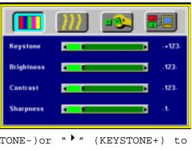
Press the "Menu" key again to enter Display page items, or press " (KEYSTONE-)or " (KEYSTONE+) to select sub-pages. (The main OSD menu will automatically disappear if a key is not pressed within 10 seconds). Figure 21 Main OSD menu Press the "Exit" (AUTO) button to leave the current sub-page, and press "Exit" (AUTO) the button again to leave the main OSD menu (at the same time the settings are saved).
