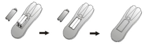
Figure 15 Battery replacement process
